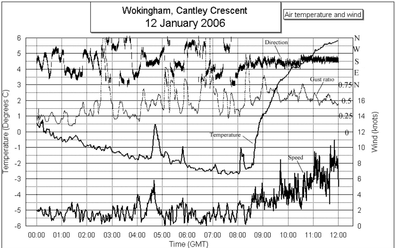
Fig1. Graph of temperature and wind for 12 January 2006, 00 to 12 GMT, Wokingham Cantley Crescent. The four parameters plotted are: 1) temperature, one minute average from aspirated psychrometer, 2) wind speed, 1 minute average from sonic anemometer at 8 metres, 3) wind direction, one minute average, 4) 10 minute average of normalised gust ratio, (max 3 sec gust per minute minus one minute average divided by one minute average).
